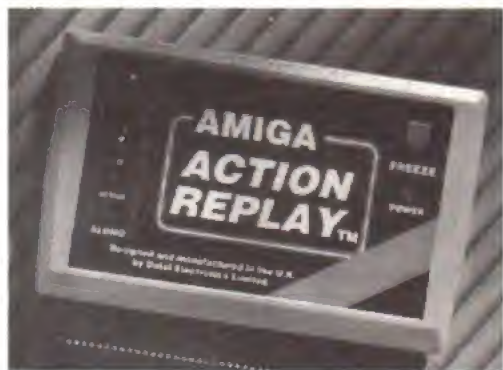
Although extremely useful for looking at programs while they're working, the Action Replay II is not very good at backing-up software.
